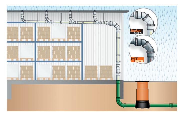
The stability and functionality of interior rainwater drainage must be guaranteed by a secure connection (DIN EN 12056-3). Wastewater pipes installed in the building are exposed to greater internal pressures due to certain loads (e.g. the rainwater drainage pipe during heavy rainfall), such as, for example:
